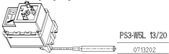
The capillary on the drawing is short just to make the picture simple. In reality it is 1 m long.
