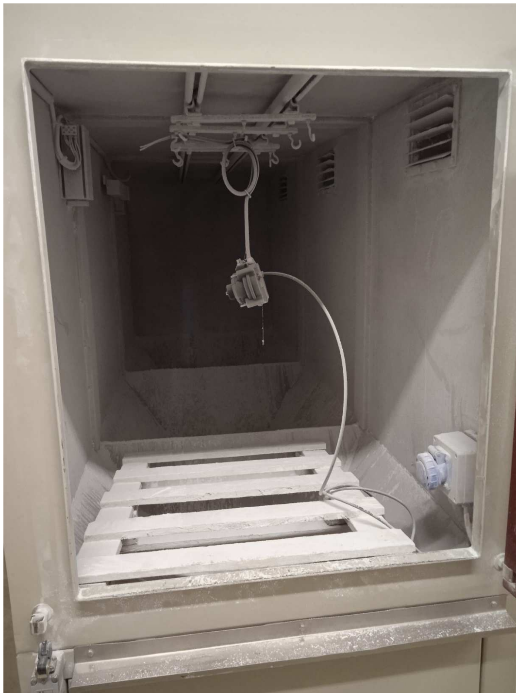
Figure 1: The EUT inside the dust chamber: a) before and b) after the IP6X
