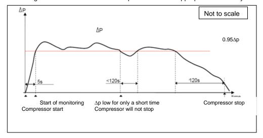
Figure 1: Functional graph using pressure differential x time axes
