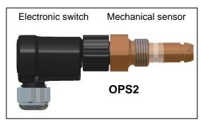
The OPS2 monitors the oil pressure differential protecting the compressor against damage if the oil differential becomes too low. Internal channels drilled through the housing link the switch to the inlet and outlet ports of the oil pump.
