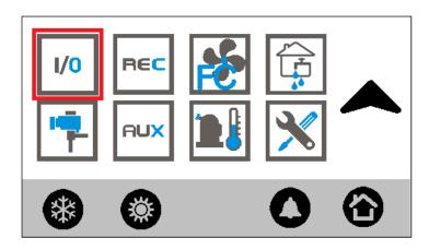
This menu allows to display the status of all inputs and outputs that have been defined.
