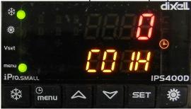
First line: Compressor/pump working hours (unit in 10 hours)
