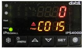
First line: Compressor starts number (unit in 10 times)
