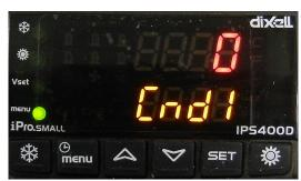
First line: Condensation fan output value.
