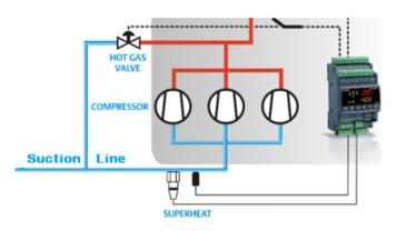
To detect the suction superheat an auxiliary probe among P3 (term. 38-42) or P4 (term. 22-23) has to be set as superheat temperature probe.
