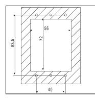
Keyboard **VC660** shall be mounted on vertical panel, in a 72x56 mm hole, and fixed using screws  $\emptyset$  3 x 2mm. To obtain an IP65 protection grade use the front panel rubber gasket (mod. RGW-V).
