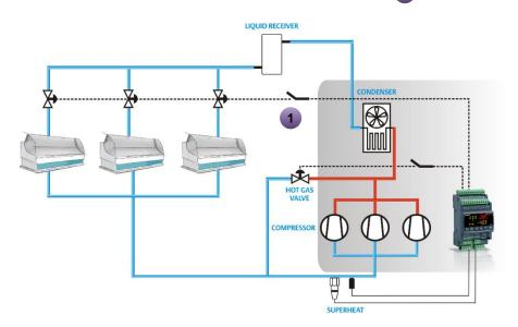
To enable this function set one relay by the parameters **oA2** or **oA3** or **oA4**, as flood protection, El **oA4 = Liq**, and then connect it to the external device that blocks the cabinet injection. NOTE: the relay set as flood protection is automatically activated even when the controller is in stand-by mode.
