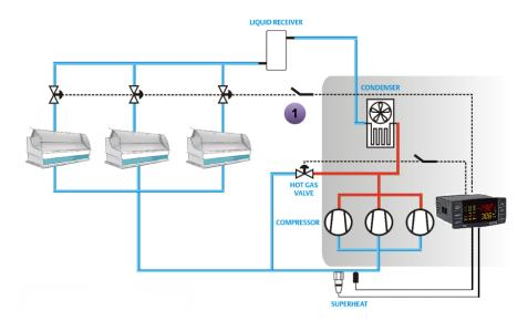
To enable this function set one relay by the parameters **oA2** or **oA4** or **oA5** or **oA6**, as flood protection, EI **oA4 = Liq**, and then connect it to the external device that blocks the cabinet injection.
