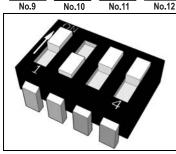
The address is set in binary mode. Every selector has a different weight, in figure nearby the address is:
